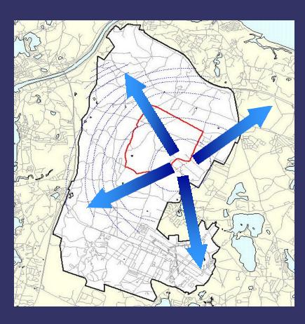
Groundwater flow is radial with the mound to the southeast of the Impact Area Groundwater flow is approximately one foot per day
