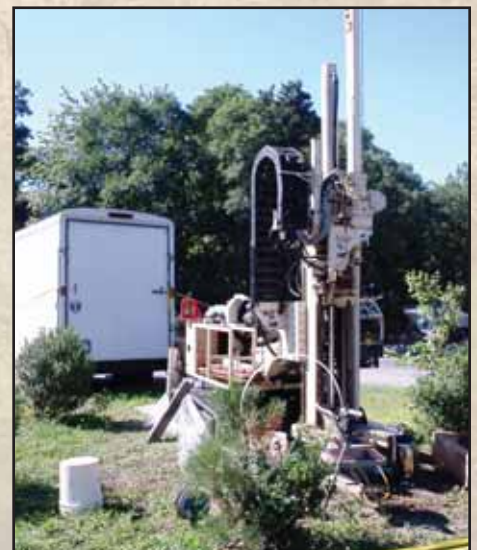
A drive-point drill rig is used to collect groundwater samples.
