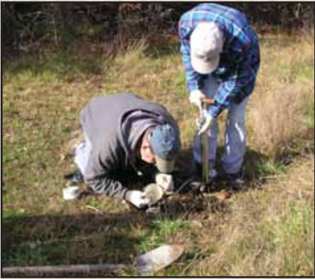
Water is sampled using a shallow water-capture system known as a lysimeter.
