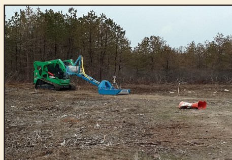
The Metal Mapper is used to discriminate between buried unexploded ordnance items and other non-hazardous metallic objects in the Central Impact Area.
