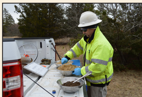
Soil samples from a source area being processed for shipping and testing.
