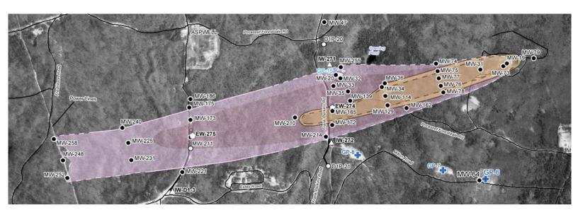
The Rapid Response Action extraction, treatment and reinjection systems at Frank Perkins and Pew Roads, shown by white dots, will continue to operate as part of Alternatives 2-6. (Contour lines dashed where inferred.)
